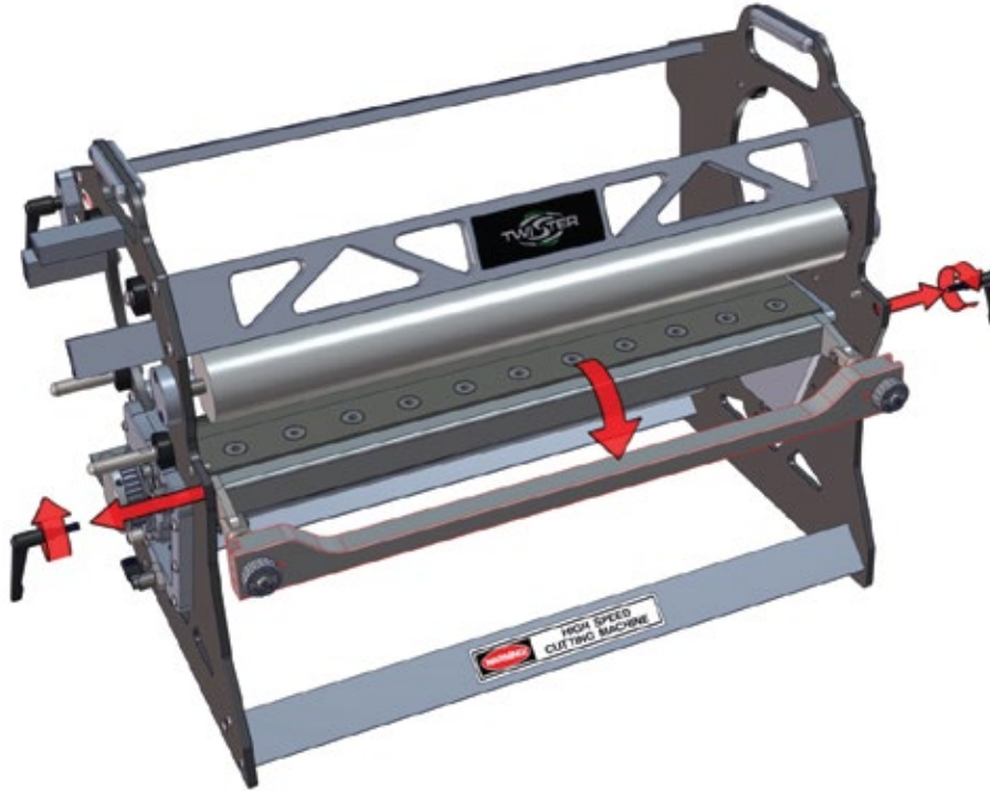
Figure 29: Unlocking the adjuster crossbar
