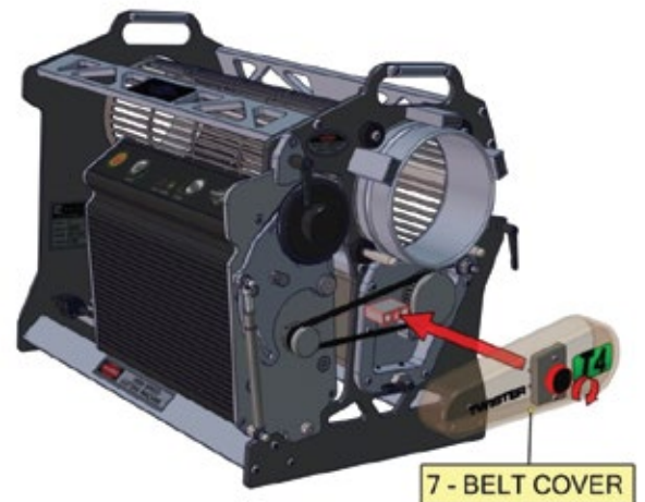
Figure 4: Installing the belt cover
