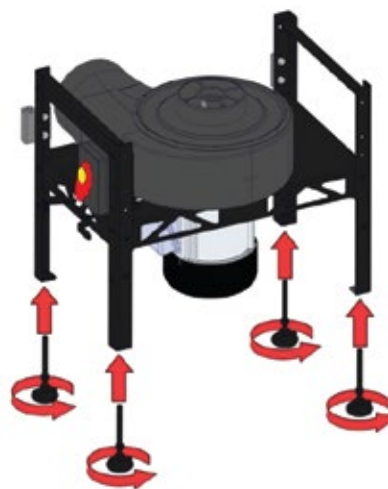
Figure 10: Installing feet on the leaf collector
