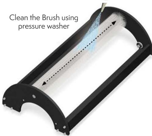
Clean the length of the CUTTING REEL and SHROUD of all debris
