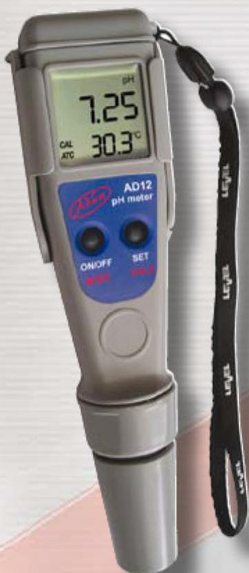
AD11 and AD12 are the most advanced microprocessor based Waterproof pH/Temp pocket testers in the market.
