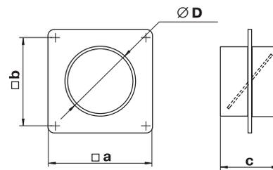
Connector with plate for round ducts
